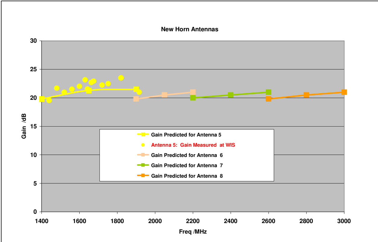
Figure 13: Antenna gains predicted (gain for horn antenna 5 vs. at WIS measured gain)
